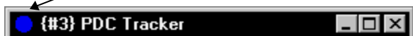
Figure 46 Title Bar Right-click on the symbol to open the Properties dialog box.
